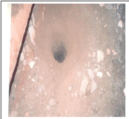
Auger Boring for Sampling
